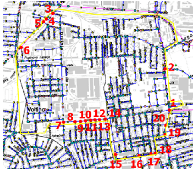
A DMA/PMA zone with marked peripheral chambers in which boundary valves will be closed
