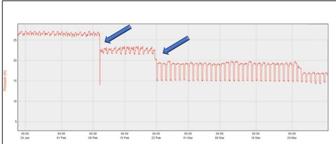
FIGURE F-16 Example of pressure configuration error
