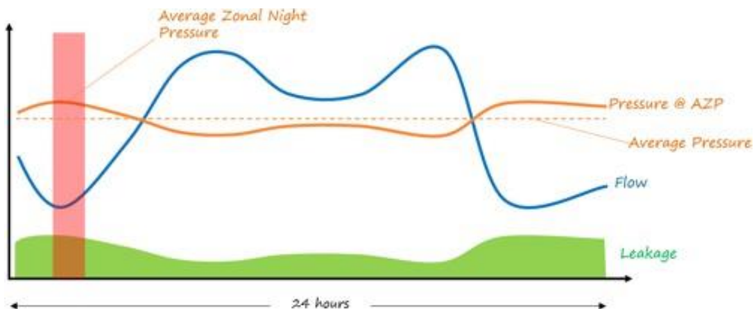
FIGURE E-5 AZP Pressure & Leakage Illustration.
