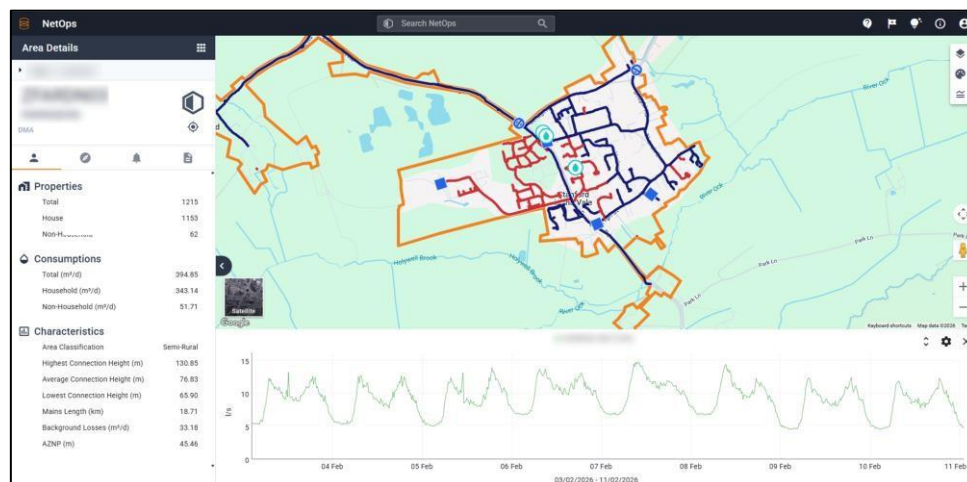
Figure 6-1 Example of a dashboard of DMA Data Management System (source: Crowder Consulting).
