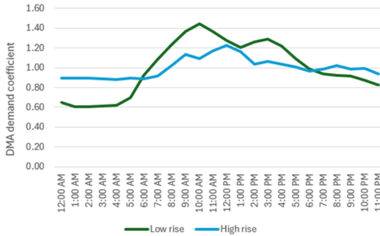
Figure 4-6 Difference in flow pattern due to presence of storage tanks (source: WMI, 2019)
