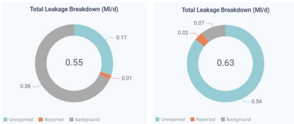
Figure 5-1 Breakdown of Total Leakage in Example DMAs.
