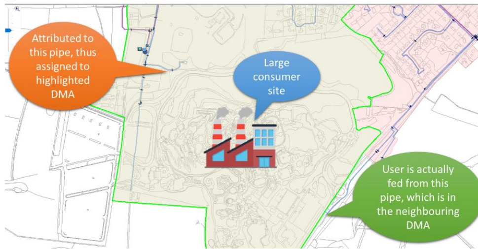
FIGURE F-20 Example of customer DMA assignment error
