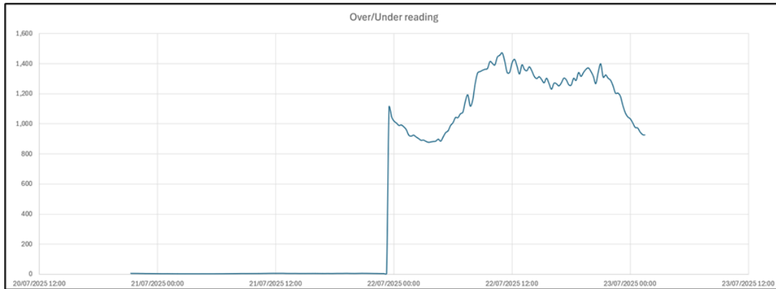
FIGURE F-13 Example of flow signal with a logger calibration problem
